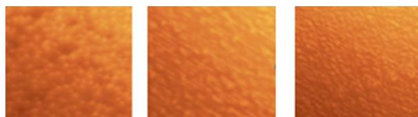
**Figure 2** Surface morphology of CdS thin films, deposited from solution with pH = 6.7 (a), pH = 9.5 (b), and pH = 10.2 (c).
