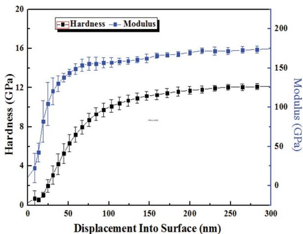
**Figure 5.** Evolution of the hardness and elastic modulus as a function of indentation depth for the Cr/GLC film.
