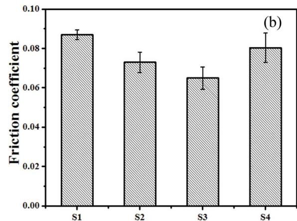
**Figure 6.** Friction curves and average friction coefficient of the patterned Cr/GLC films under seawater.
