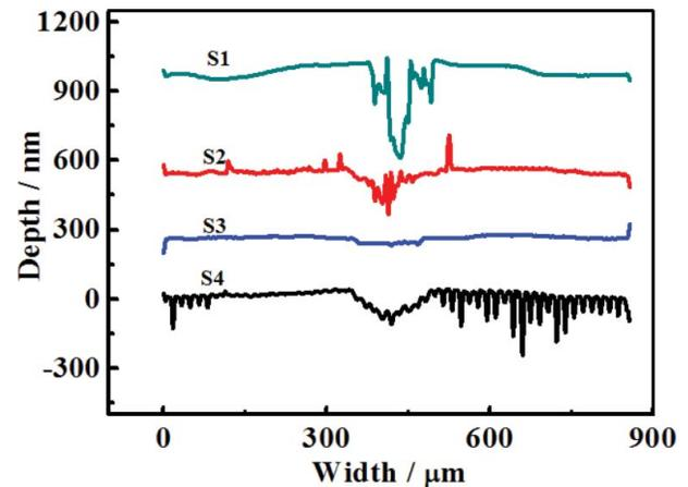
Figure 8. 2D cross-section profiles of the wear tracks on the patterned Cr/GLC films in seawater.
