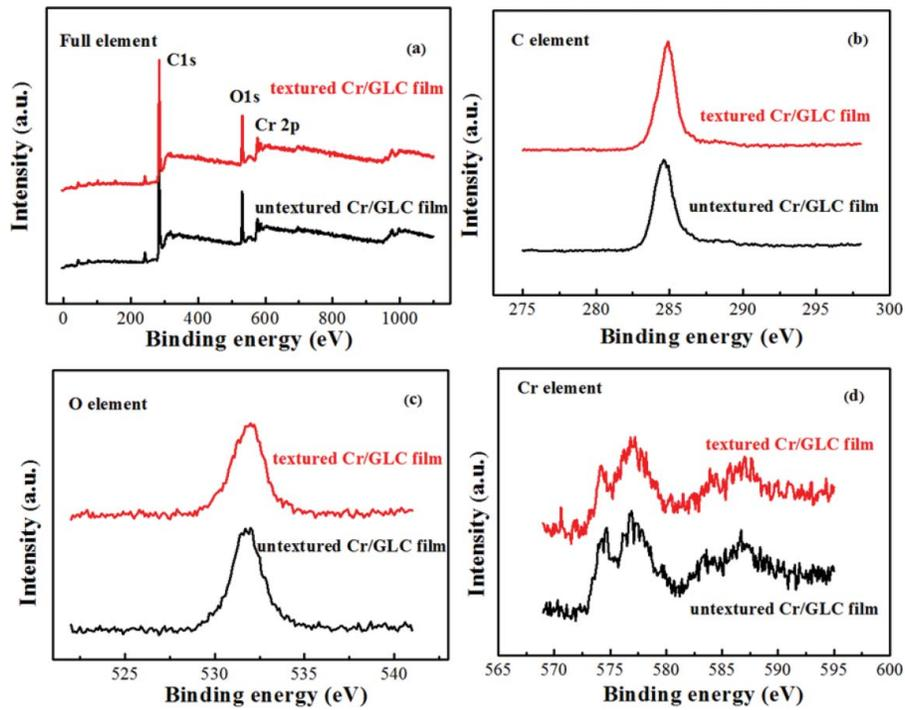
**Figure 3.** XPS spectra of (a) full element, (b) C1s, (c) O1s, and (d) Cr2p of the Cr/GLC films with different micro/nanotextures.
