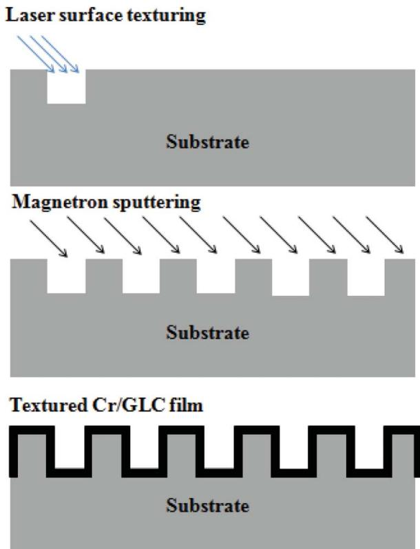
Figure 1. Schematic illustration of the process of producing textured Cr/GLC films.
