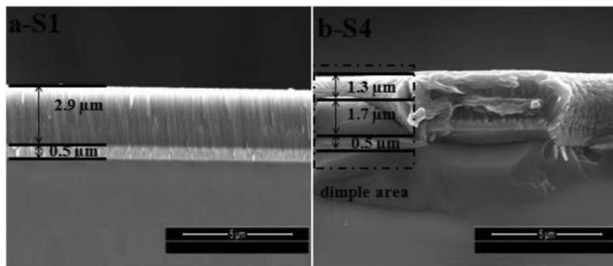
**Figure 4.** Cross-section morphologies of the S1 and S4 films.
