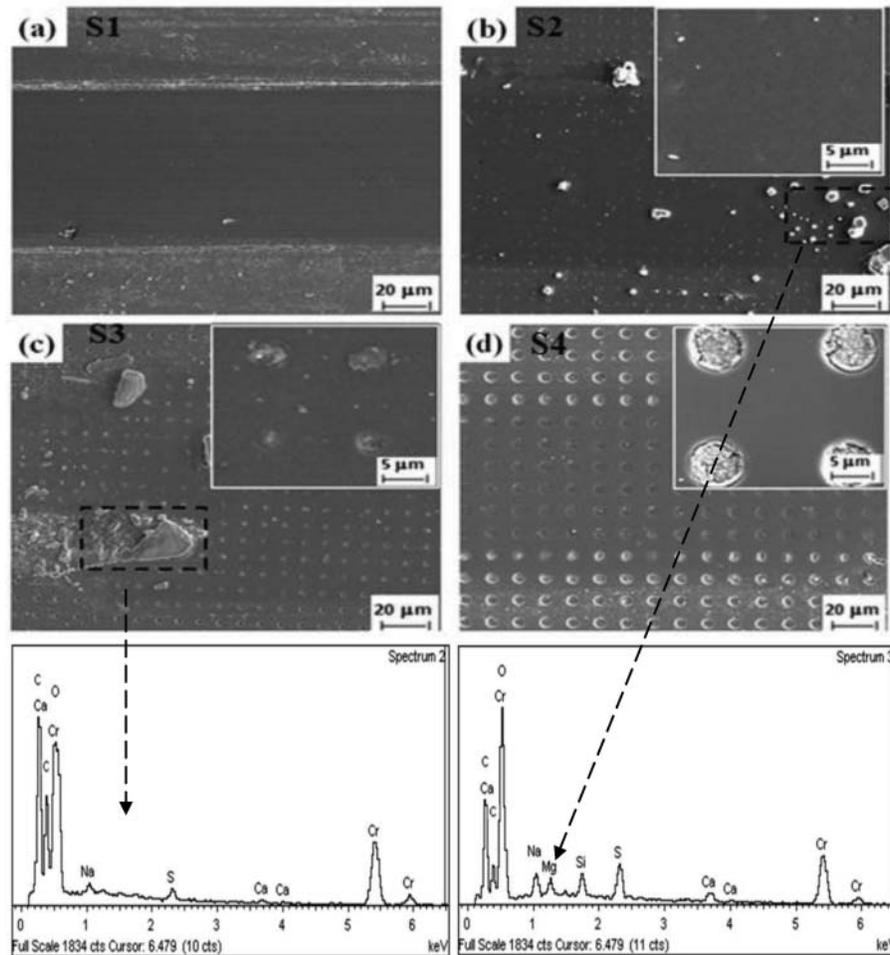
**Figure 9.** Morphologies of the wear tracks on the patterned Cr/GLC films in seawater.
