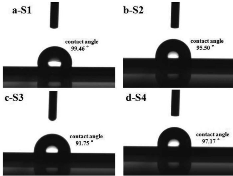
Figure 11. Effect of surface texture on the contact angle of the patterned Cr/GLC films.
