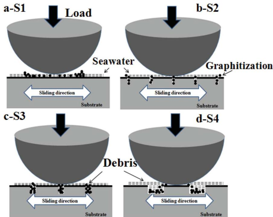
**Figure 12.** Cross-sectional schematic view of the wear mechanism model for (a) S1, (b) S2, (c) S3, and (d) S4.
