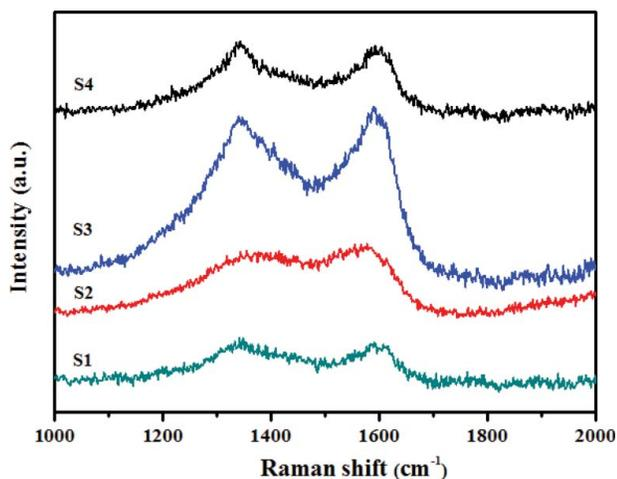
**Figure 10.** Raman spectra obtained from the contact surface of the WC ball.
