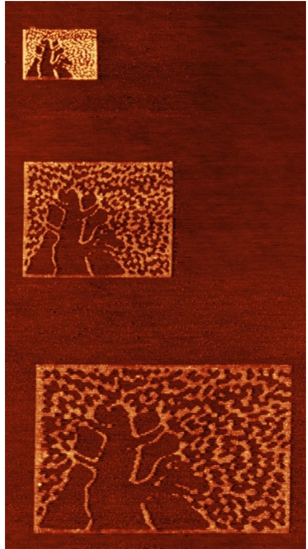
Raster voltage lithography on organic monolayer at different scale (from bottom to top 2x1.5, 4x3, 7x5 microns). 18 x 15 microns total scan.
