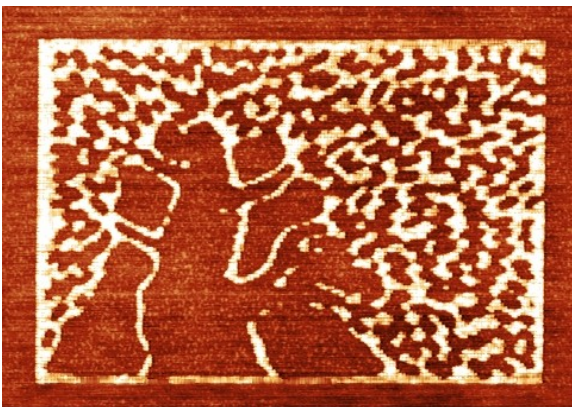
Weizmann Tree Raster voltage lithography on organic monolayer. Semi-Contact Mode, amplitude ~1nm. +15 V to sample. 5 x 8 microns scan.
